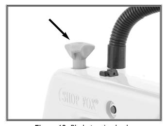
Figure 10. Blade tension knob.
